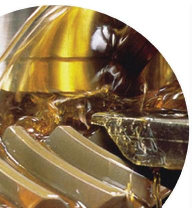
important role in machining and grinding operations? Use a low viscosity oil for high speed applications, to include grinding, and for applications wherein good chip-flushing ability is preferred. On the other hand, use a high viscosity oil for applications with low-speeds and very high depth of cuts, such as Broaching, Hobbing, and other Gear-making Operations.
