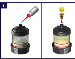
To install, fill oil into the empty unit. Open the protector and insert the NRV (Non Return Valve) to the filled unit.
