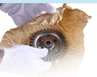
The use of Volatile Corrosion Inhibitors or VCI's, applied to paper and plastic products, have been gaining a strong following in recent years, and in most cases, the VCI products have been used as a suitable alternative for oil-based anti-rust coatings.
